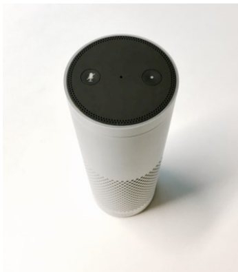
Figure 2. Amazon Echo, a standalone commercially-available device that can only be interacted with by talking to the inbuilt conversational agent Alexa. Configuration for the Echo occurs either through a smartphone app or website.
