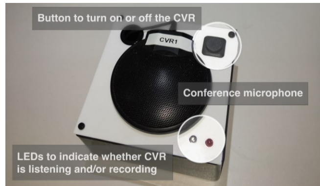
Figure 1. Conditional Voice Recorder (CVR).
